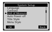
From Unit of Measure menu, use UP/DOWN scroll button to select the desired unit of measurement
