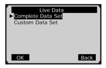
3) Use **UP/DOWN** scroll button to select a test, and press **OK** button.
