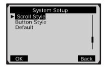
2) From **Scroll Style** menu, use **UP/DOWN** button to select scroll style between **Scroll** and **Normal**.
